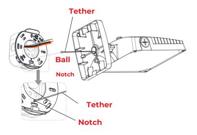
Secure the tether ball into the mounting plate notch to help with handsfree wiring.
