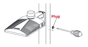
Using the screwdriver, unscrew the plug from the side of the luminaire.
