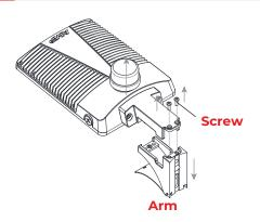
Remove the top (2) screws as shown to remove the arm from the luminaire.
