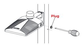
Using the screwdriver, thread previously removed waterproof screw back onto the side of the luminaire. Hand tighten until snug.
