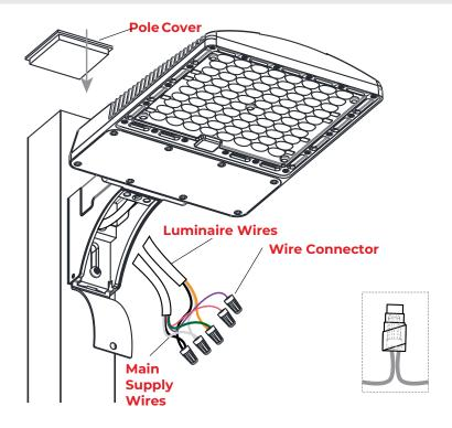
Feed the supply wires and luminaire wires into the arm wiring compartment. Make the connections as follows:
