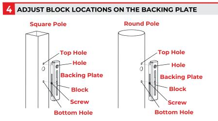
Insert and hold the backing plate into the pole.
