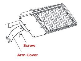
Access the wiring compartment by removing the screw from the arm cover.
