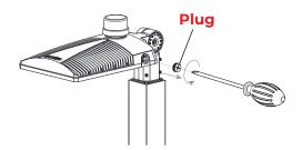
Remove threaded Plug from the side of the luminaire to access the selection switches.
