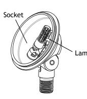
Insert the lamp with the correct wattage and type marked on the luminaire label.
