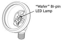
NOTE: "Wafer" bi-pin LED lamp also can be used for this luminaire.
