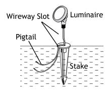
Clear away an area in the ground at the wireway slot on top of the stake. Align the wireway slot on the base of the stake. Lay the luminaire pigtail into the wireway slot and screw the luminaire onto the stake. Tighten until snug to secure the base.
