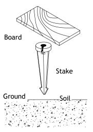
Determine the desired location for mounting the stake mount. Hammer the stake into the ground until flange of stake is flush to grade. To avoid damage to the stake, place a board on top of the stake while hammering.
