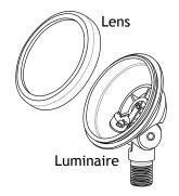
Loosen the lens and remove it from the luminaire.
