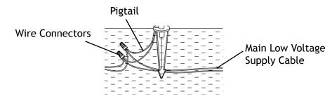
Strip both leads from the luminaire pigtail. Using two wire connectors (sold seperatley), connect the leads from the luminaire to the main low voltage supply cable leads.
