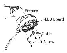
Loosen the screws, and remove the optic from the fixture.
