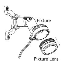
Turn the fixture lens counterclocwise and remove it from the fixture.
