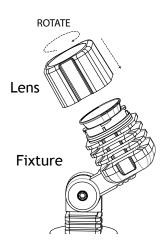
Place the lens back onto the fixture and rotate it until it is secured properly.
