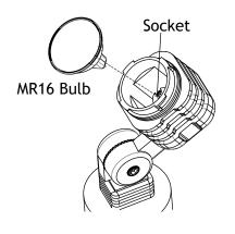
Insert MR16 bulb with the correct wattage and type marked on the fixture label.
