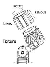
Rotate the lens to remove it from the fixture.
