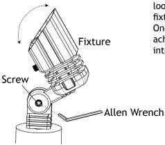
Using the provided Allen wrench, loosen the knuckle and adjust the fixture to your desired direction. Once your desired direction is achieved, tighten the knuckle into place.
