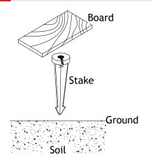
Determine the desired location for mounting the stake mount. Hammer the stake into the ground until flange of stake is flush to grade. To avoid damage to the stake, place a board on top of the stake while harmmering.
