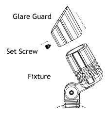
Install the glare guard back onto the fixture and secure with previously removed set screw.
