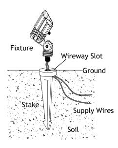
Clear away an area in the ground at the wireway slot on top of the stake. Lay the fixture pigtail into the wireway slot and attach the fixture onto the stake. Tighten until snug.
