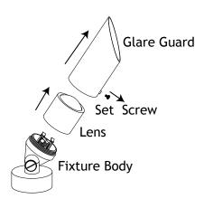
Loosen the lens and the set screw and remove the glare guard.
