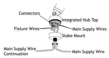
Insert the main supply wire continuation (if needed) and the main supply wire up through the bottom of the stake mount and strip the ends of both sets of supply wires.
