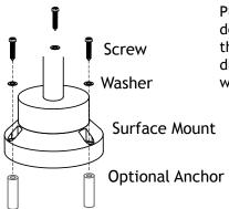
Place the surface mount onto the desired location and secure it with the screws. Tighten with a screwdriver. Nylon spacers are required when installing on trees.
