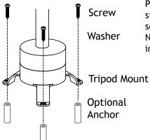
Place the tripod mount onto the desired location and secure it with the screws. Tighten with a screwdriver. Nylon spacers are required when installing on trees.
