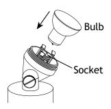
Insert the bulb with the correct wattage and type marked on the luminaire label.
