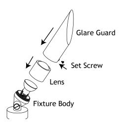
Thread the lens onto the fixture body and hand tighten.
