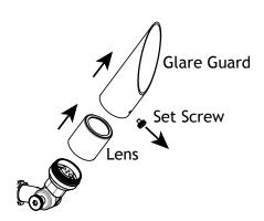
Loosen the set screw on the glare guard and remove it from the lens. Then twist and remove the lens from the fixture.
