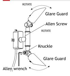
Using an Allen wrench, loosen the knuckle and adjust the fixture up and down to your desired direction.
