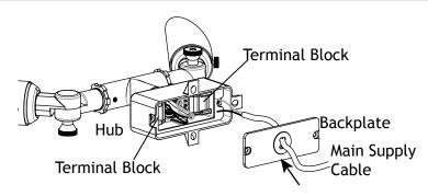
Pass the main supply cable through the center hole on the backplate.
