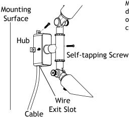
Make sure the wire exit is facing down on the hub, then attach it onto the mounting surface and secure with the self-tapping screws.
