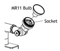
Insert the MR11 bulb with correct wattage and type marked on fixture label and secure into place. CAUTION: Do not exceed maximum wattage marked on luminaire label.
