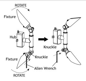
Using an Allen wrench, loosen the knuckles to rotate the fixtures as shown.
