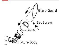
Thread the lens back onto the fixture body and hand tighten until snug.
