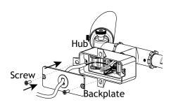
Carefully tuck all the extra wire inside of the hub and place the backplate onto the hub. Secure by using the previously removed screws. Tighten with a screwdriver.
