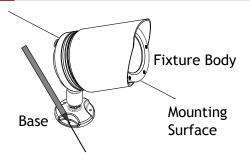
Mark three points on the mounting surface using the holes on the base as guides. These marks will be used for anchors.
