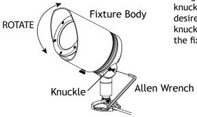
Using the Allen wrench, loosen the knuckle to adjust the fixture to the desired orientation. Tighten the knuckle with the Allen key to secure the fixtures adjustment.
