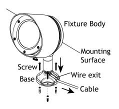
Place the base onto the anchors and secure with screws.
