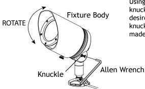
Using Allen wrench, loosen the knuckle to adjust the fixture to the desired orientation. Tighten the knuckle after the adjustments are made.
