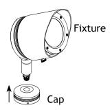
Thread the cap onto the fixture body and hand tighten until snug.
