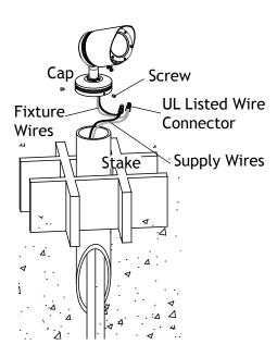
Allow enough wire from the fixture for adjustment purposes. Strip both leads from the fixture pigtail. Using two UL listed wire connectors (sold separately), connect the leads from the fixture to the main supply cable leads. Place the wire into the stake and attach the cap back onto the stake using the screws.
