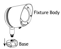
Unscrew the base and remove it from the fixture body.
