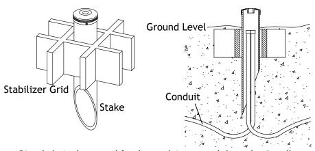
Dig a hole in the ground for the conduit runs and the stake. Install the conduit. Slide the stabilizer grid onto the stake and secure with the screws. Place the stake over the conduit runs. Backfill against the mounting stake.
