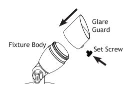
Place the glare guard back onto the fixture body and secure with the previously removed set screw. Hand tighten until snug.
