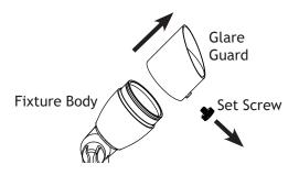
Loosen the set screw to remove the glare guard from the fixture body.
