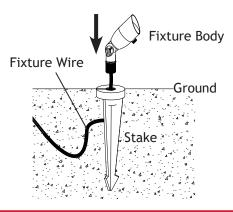
Pass the fixture wire through the center hole of the stake. Thread the fixture body onto the stake and hand tighten until snug.
