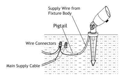
Strip both leads from the fixture body. Using two wire connectors (sold separately), connect the leads from the fixture body to the main supply cable leads.
