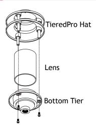
Loosen the screws from the bottom of the TieredPro Hat. Remove the bottom tier to expose the lens and replace it with the new replacement shade. Reinstall the bottom tier to hold the shade and secure it with the screws removed previously. Tighten until snug.
