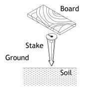
Determine the desired location for mounting the luminaire. Hammer the stake into the ground until flange of stake is flush to grade. To avoid damage to the stake, place a board on top of the stake while hammering.
