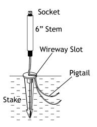
Clear away an area in the ground at the wireway slot on top of the stake. Lay the luminaire pigtail into the wireway slot and screw the stem onto the stake. If the fixture does not look straight, adjust by pushing or pulling on the stake only.
