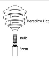
Place the TieredPro hat over the bulb and thread onto the top end of the stem. Hand tighten until snug.
