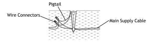
Strip both leads from the luminaire pigtail. Using two wire connectors (sold separately), connect the leads from the luminaire to the main low voltage supply cable leads.
