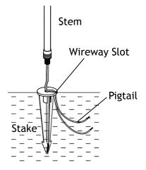
Clear away an area in the ground at the wireway slot on the top of the stake. Lay the luminaire pigtail into the wireway slot and secure the stem onto the stake. If the fixture does not look straight, adjust by pushing or pulling on the stake only.
