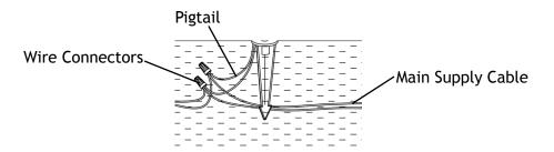
Strip both of the leads from the luminaire pigtail. Using two wire connectors (sold separately), connect the leads from the luminaire to the leads of the main supply cable.
