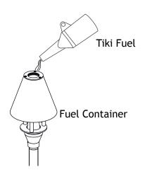
Pour tiki fuel in the fixture's fuel container as shown. Never use gasoline, kerosene, or other flammable fuels.
