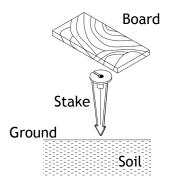
Determine the desired location for mounting the luminaire. Hammer the stake into the ground until flange of stake is flush to grade. To avoid damage to the stake, place a board on top of the stake while hammering.
