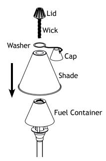
Place the shade and the washer back onto the container. Insert the wick inside of the fuel container and tighten the lid until snug. Put the cap back onto the top end of the fixture over the lid. Before lighting the torch insure that the wick is completely saturated.
