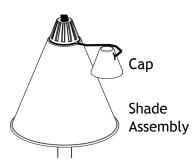
Remove the cap from the top end of the shade assembly.
