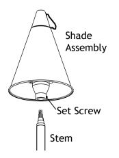
Attach the shade assembly onto the top end of the stem as shown. Tighten the set screw until snug to secure both pieces together.
