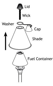
Remove the washer with the cap and the shade from the fuel container by unscrewing the lid.
