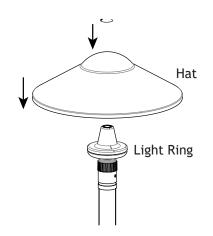
Thread the hat of your choice onto the stem top. Hand tighten until snug.
