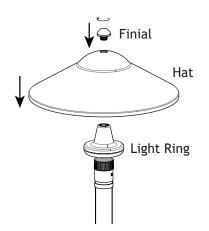
Remove the finial from the light ring first. Place the hat of your choice onto the light ring and secure with the finial. Hand tighten until snug.
