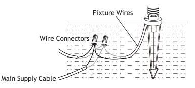
Strip both leads from the fixture wires. Using two UL listed wire connectors (sold separately), connect the leads from the fixture wires to the main supply cable leads.
