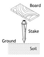
Determine the desired location for mounting the luminaire. Hammer the stake into the ground until the flange of stake is flush to grade. To avoid damage to the stake, place a board on top of stake while hammering.
