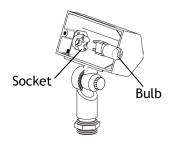
Insert the bulb with correct wattage and type marked on the luminaire label.
