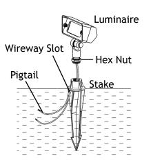
Clear away an area in the ground at the wireway slot on top of the stake. Lay the luminaire pigtail into the wireway slot and screw the fixture on to the stake. Tighten the hex nut on the luminaire against the stake and tighten until snug.
