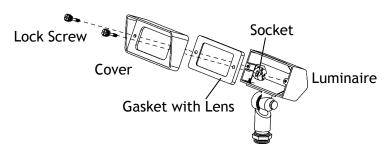
Loosen the lock screws and remove the cover and gasket with the lens from the luminaire to expose the socket.
