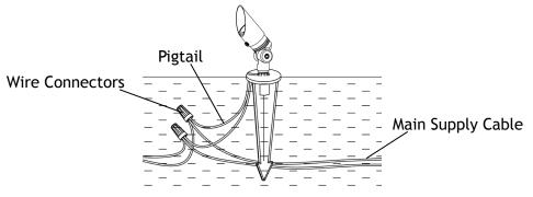
Strip both leads from the luminaire pigtail. Using two wire connectors (sold separately), connect the leads from the luminaire to the main supply cable leads.
