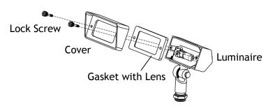
Decide which lens you would like to use with this fixture. Then install the gasket with your lens of choice back onto the luminaire and secure with the lock screws.
