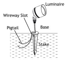
Clear away an area in the ground at the wireway slot on top of the stake. Lay luminaire pigtail into the wireway slot and secure the fixture onto the stake. Tighten until snug.
