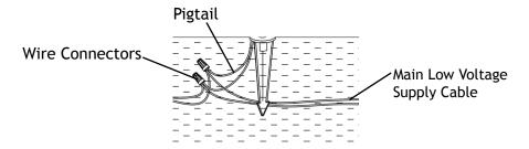
Strip both leads from the luminaire pigtail. Using two wire connectors (sold separately), connect the leads from the luminaire to the main low voltage supply cable leads.
