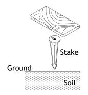
Determine the desired location for mounting the fixture. Hammer the stake into the ground until flange of stake is flush to grade. To avoid damage to the stake, place a board on top of stake while hammering.
