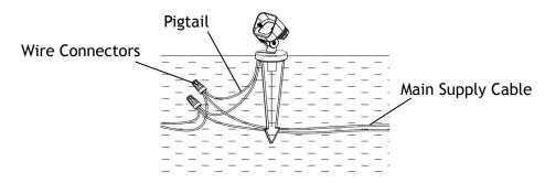
Strip both leads from the luminaire pigtail. Using two wire connectors (sold seperately), connect the leads from the luminaire to the main supply cable leads.
