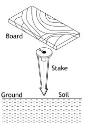
Determine the desired location for mounting the luminaire. Hammer the stake into the ground until flange of stake is flush to grade. To avoid damage to the stake, place a board on top of the stake while hammering.
