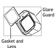
Remove the lens from the rubber gasket, then replace it with the lens you would like to use.
