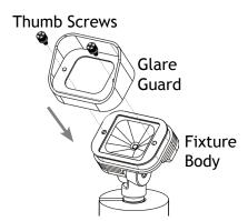
Place the glare guard and the gasketed lens back onto the fixture body and secure with the thumb screws previously removed. Hand tighten until snug.
