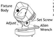
Use the included Allen wrench to unlock the set screw and adjust the fixture body to your desired direction. Tighten the set screw once your desired angle is achieved.
