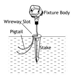
Clear away an area on the ground at the wireway slot on top of the stake. Lay the luminaire pigtail into the wireway slot and thread the fixture onto the stake. Tighten using the lock nut to secure it to the base.
