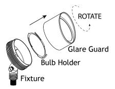
Rotate the glare guard counter clockwise and remove it from the fixture. Then remove the bulb holder.
