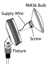
Use a PAR36 bulb (sold separately), with the correct wattage and type as marked on luminaire label. Connect the supply wires using the screws on the bottom of the PAR36 bulb, tighten with a screwdriver.
