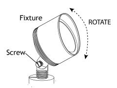
Loosen the knuckle and adjust the fixture to the desired orientation. Tighten the knuckle after you find the desired orientation.
