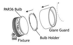
Tuck the excess wires inside of the fixture and place the PAR36 bulb inside. Place the bulb holder onto the top of the PAR36 bulb and thread the glare guard onto the fixture.
