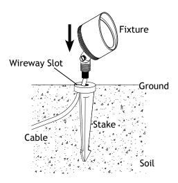
Clear away an area in the ground at the wireway slot on the top of the stake. Place the fixture wire into the wireway slot and thread the fixture onto the stake. Hand tighten until snug.
