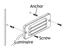
Note: Anchors are required for concrete or brick walls. Hold the luminaire on the wall and mark two points for the anchors using the mounting holes as guides. Then drill the proper holes using the marks. Insert the anchors into the drilled holes.
