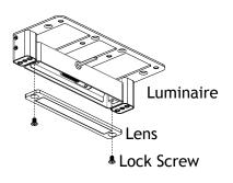
Install the lens back onto the luminaire and tighten with previously removed lock screws.
