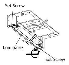
Using an Allen Key, loosen the set screws on the side of the fixture to rotate the luminaire to your desired direction by hand. Once you have the desired angle, tighten down the set screws with the Allen Key.
