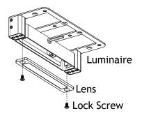
Remove the lens from the luminaire by loosening the lock screws.
