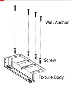
Place the fixture body onto the desired location. Mark four points on the mounting surface using the holes of the mount as a guide. Set the fixture aside and drill the proper holes where you placed the marks then insert the wall anchors into the drilled holes.
