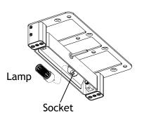
Insert lamp with the correct wattage and type marked on the fixture label and push firmly into place.
