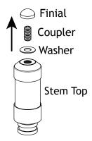
Loosen the finial and remove the finial, coupler and washer from the stem top.
