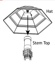
Thread the hat onto the stem top and hand tighten until snug.
