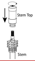
Place the stem top over the lamp and thread the stem top onto the stem. Hand tighten until snug.
