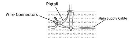
Strip both leads from the luminaire. Using two wire connectors (sold separately), connect the leads from the fixture to the main supply cable leads.
