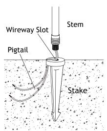
Clear away an area in the ground at the wireway slot on top of the stake. Lay the luminaire pigtail into the wireway slot and secure the stem onto the stake. Tighten until snug.
