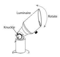
Loosen the knuckle to adjust the luminaire to your desired direction. Always tighten the knuckle once your desired direction is achieved.
