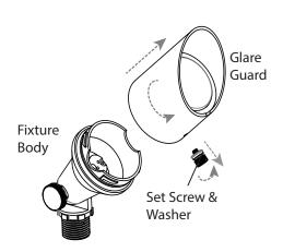
Place the glare guard back onto the fixture body and rotate it clockwise. Thread the set screw with washer back onto the glare quard.
