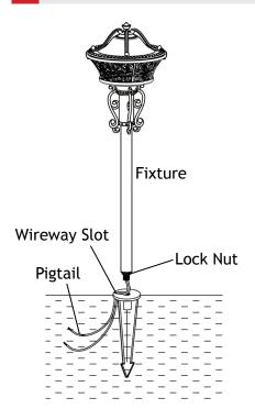
Clear away an area in the ground at the wireway slot on top of the stake. Lay the luminaire pigtail into the wireway slot and thread the fixture onto the stake.
