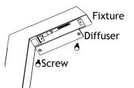
Attach the diffuser back onto the fixture and secure with screws. Tighten until snug.
