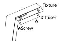
Remove the diffuser from the fixture by unthreading the screws.
