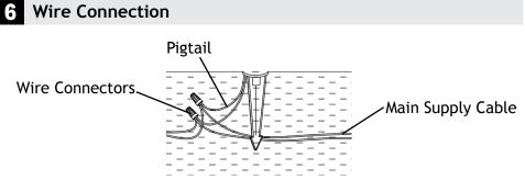
Strip both leads from the luminaire pigtail. Using two wire connectors (sold separately), connect the leads from the luminaire to the main low voltage supply cable leads.
