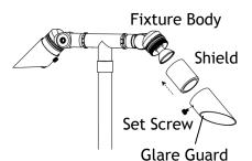
Place the shield over the lamp and thread onto the fixture. Attach the glare guard back onto the shield and secure with the set screw. Tighten until snug.
