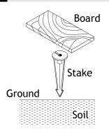
Determine the desired location for mounting the fixture. Hammer the stake into the ground until flange of stake is flush to grade. To avoid damage to the stake, place a board on top of the stake while hammering.
