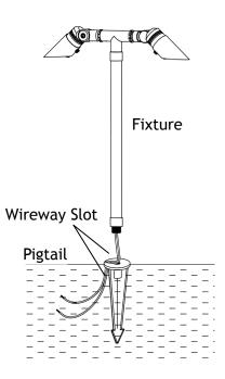
Clear away an area in the ground at the wireway slot on top of the stake. Align the wireway slot of the stake cover and the stake. Lay the luminaire pigtail into the wireway slot and attach the fixture onto the stake.
