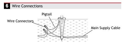
Strip both leads from the luminaire pigtail. Using two wire connectors (sold separately), connect the leads from the luminaire to the main supply cable leads.
