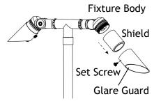
Loosen the set screw and remove the glare guard from the shield. Remove the shield from the fixture.
