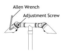
Using an Allen Wrench, loosen the adjustment screws and modify the fixture bodies to the desired angles. Then tighten the adjustment screws.
