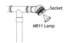
Insert the lamp with the correct wattage and type marked on the fixture label.
