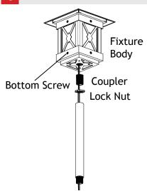
Using a screwdriver, remove the bottom 4 screws from the fixture body. Pull the lead wire into the center of the fixture through the side wire exit and then place it through the center hole going back out. Attach the bottom back onto the fixture body and secure with the previously removed screws.
