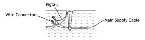
Strip both leads from the luminaire pigtail. Using two wire connectors (sold separately), connect the leads from the luminaire to the main supply cable leads.
