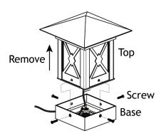
Using a screwdriver, unscew the screws on the side of the base and remove the top from the base.
