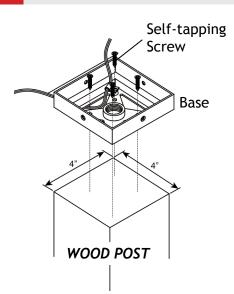
Attach the base onto a 4" x 4" square wood post and secure with the self-tapping screws. Hand tighten with a screwdriver.
