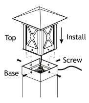
Attach the top back onto the base and secure with the screws previously removed. Hand tighten with a screwdriver.
