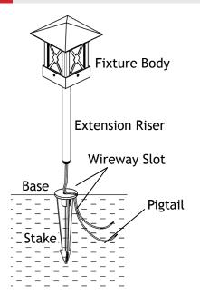
Clear away an area in the ground at the wireway slot on top of the stake. Lay the luminaire pigtail into the wireway slot. Then, thread the bottom end of the extension riser with the fixture body onto the stake. Tighten to secure the base.
