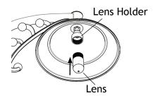
Thread the lens back onto the lens holder and hand tighten.
