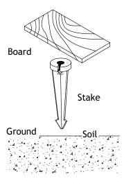
Determine the desired location for mounting the stake mount. Hammer the stake into the ground until flange of stake is flush to grade. To avoid damage to the stake, place a board on top of the stake while hammering.
