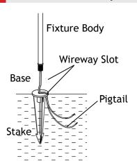
Clear away an area in the ground at the wireway slot on top of the stake. Lay the luminaire pigtail into the wireway slot and thread the coupler onto the stake. Tighten to secure the base.
