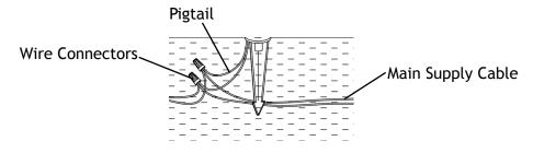
Strip both leads from the luminaire pigtail. Using two wire connectors (sold separaetly), connect the leads from the luminaire to the main supply cable leads.
