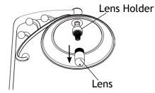
Loosen the lens from the lens holder to expose the socket.
