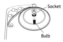
Insert the bulb with the correct wattage and type marked on the fixture label.
