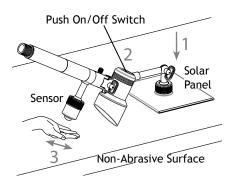
Place the solar light on a nonabrasive surface with the solar panel face down. Press the ON/OFF switch on the back of the fixture body. Wave your hand in front of the sensor to test the fixture.
