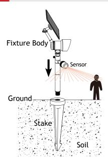
Thread the fixture body on to the stake. Hand tighten until snug. Make sure the sensor is facing the desired area to be monitored during installation.
