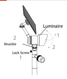
Adjust the sensor by using the lock screw.
