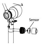
If necessary, remove the cover to replace the sensor. Always install the cover back to protect the sensor.
