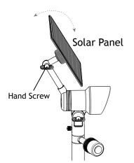
Adjust the solar panel piece forward and backwards by using the hand screw. You can also take the solar panel piece itself and rotate it in any direction you need to face the sun.
