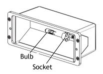
Insert the bulb with the correct wattage and type marked on the luminaire label.
