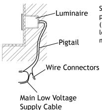
Strip both leads from the luminaire pigtail. Using two wire connectors (sold separately), connect the leads from the luminaire to the main supply cable leads.
