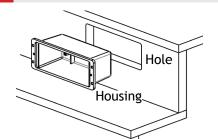
Using the luminaire housing as a template, mark the location of the housing on the wall or deck. Cut the hole from the mark.
