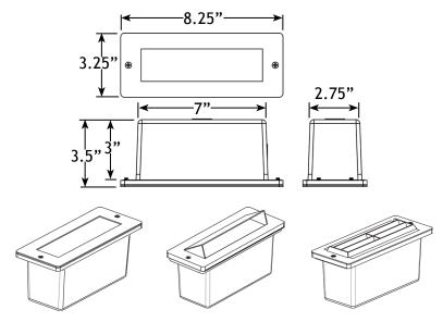
Open Face Step Light Hooded Step Light Louvered Step Light
