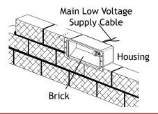
Mortar housing into place as if it were a brick.
