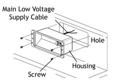
Pass the supply wires through the cut holes and insert the housing into the hole. Secure with screws.
