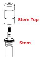
Place the stem top over the bulb and thread the stem top onto the stem. Hand tighten until snug.
