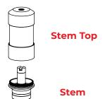
Loosen the stem top and remove it from the stem.
