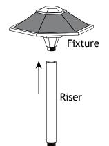
Thread the riser onto the fixture and hand tighten until snug.
