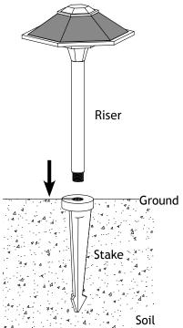
Thread the riser on to the stake and hand tighten until snug.
