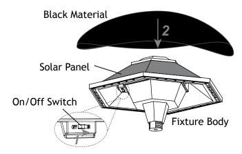
Slide the ON/OFF switch of the fixture to the "ON" position. Cover solar panels completely by using black materials. The fixture will light up when the solar panel is covered and turn back off when it is uncovered.
