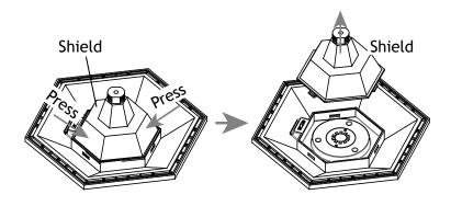
Press the sides of the shield to remove it from the fixture body.
