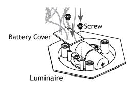
Remove the battery cover from the luminaire by using a screwdriver and removing the screws.
