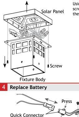
Using a screw driver, remove the screws from the corners to remove the solar panel from the fixture body.
