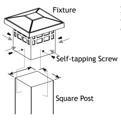
Attach the fixture onto a 4"x 4" square wood post and secure with self-tapping screws. Tighten with a screwdriver.
