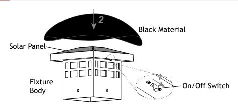
Slide the ON/OFF switch of the fixture to the "ON" position. Cover solar panels completely by using a dark material. The fixture will light up when the solar panel is covered and turn off when it is uncovered.
