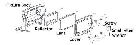
Use the Small Allen Wrench to loosen the screws on the cover to remove the cover, the lens and the reflector from the fixture body.
