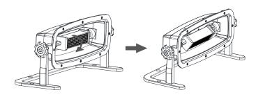
If you would like to decrease the output, rotate the R7S bulb towards the back of the fixture.
