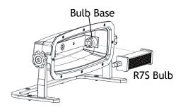
Insert the R7S bulb with the correct wattage and type marked on fixture label and push into place. Make sure the LED surface of R7S bulb is facing outside during installation.
