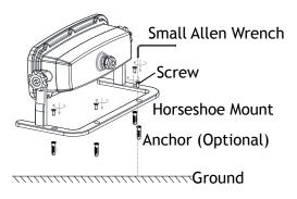
Attach the horseshoe mount to the desired location and mark (4) points for anchors from the holes on the horseshoe mount. Drill proper holes on the location and insert the anchors into the drilled holes. Attach the horseshoe mount onto the anchors. Thread the mounting screws into the anchors to secure the horseshoe mount. Hand tighten until snug with Small Allen Wrench.
