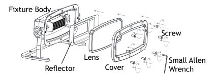
Place the reflector, the lens and the cover back onto the fixture body and secure with previously removed screws. Hand tighten until snug with Small Allen Wrench.
