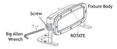
Use the Big Allen Wrench to loosen the screws on the sides to rotate the fixture body to the desired direction. Always tighten the screws after adjustment.
