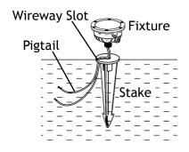
Clear away an area on the ground at the wireway slot on top of the stake. Lay the luminaire pigtail into the wireway slot and screw the fixture onto the stake. Tighten until snug.
