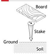
Determine the desired location for mounting the fixture. Hammer the stake into the ground until flange of stake is flush to grade. To avoid damage to the stake, place a board on top of the stake while hammering.
