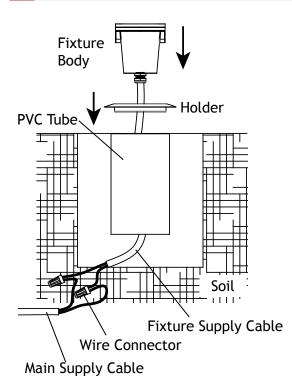
Pass the fixture supply cable through the holder and the PVC tube. Place the holder onto the PVC tube, then place the fixture body into the holder properly.
