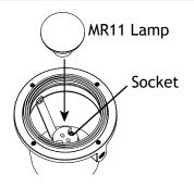
Insert the lamp with the correct wattage and type marked on the fixture label and push firmly into place.
