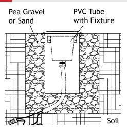
Install the PVC tube with the fixture in the hole and fill the hole with pea gravel or sand.
