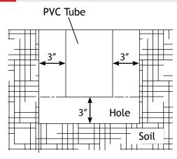
Prepare a hole in the ground. Make sure there are approximately 3" spaces surrounding the PVC tube for pea gravel or sand.
