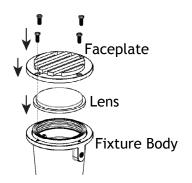
Place the lens and faceplate onto the fixture body and secure with previously removed screws in a star pattern. Hand tighten until snug with a screwdriver.
