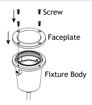
Place the lens and the faceplate back onto the fixture body and secure the removed screws in a star pattern using a screwdriver. Tighten until snug.
