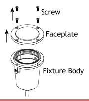
Use a screwdriver to loosen the screws on the faceplate and remove the lens from the fixture body.
