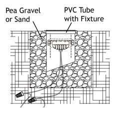
Install the PVC Tube with the fixture in the hole and fill around the fixture securing it in place with pea gravel or sand to allow for water drainage.
