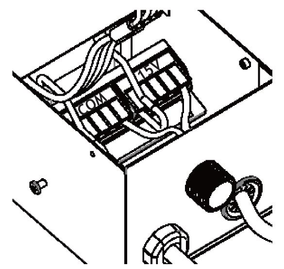
B. Run the supply wire to the centrally located hubs and insert the wire through the rubber grommets on the bottom of the hub. Then, flip one of the terminal levers open, insert one end of the stripped supply wire, and flip the lever closed to make your connection. Last, flip the lever open that is directly opposite from the first connection, on the other side of the terminal block, and insert the other end of the supply wire and flip the lever closed to make the connection.
