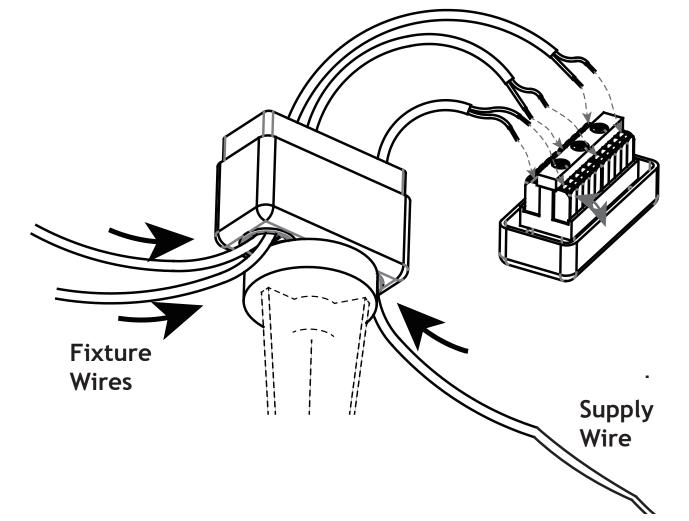
C. Run the fixture wire to the hub and insert the wire through the rubber grommets on the bottom of the hub. Then, flip one of the terminal levers open, insert one end of the stripped fixture wire, and flip the lever closed to make your connection. Last, flip the lever open that is directly opposite from the first fixture wire connection, on the other side of the terminal block, and insert the other end of the fixture wire and flip the lever closed to make the connection.
