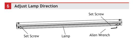
Using an Allen wrench, loosen the set screws on the ends of the lamp and then rotate the lamp to the desired direction. Always tighten the set screws after adjustments.
