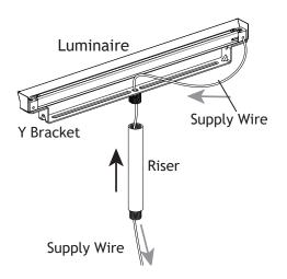
Pass the supply wire from the luminaire through the center hole on the Y bracket and the riser. Then thread the riser onto the Y bracket and hand tighten until snug.
