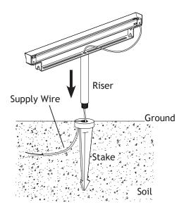
Clear away area in the ground at wireway slot on the top of the stake. Pass the fixture supply wire through the center hole of the stake and lay it into the wireway slots. Thread the riser onto the stake. Hand tighten until snug.
