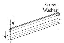
If you choose, you can attach the glare guard first before mounting the fixture.
