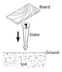
Determine the desired location for mounting the stake. Hammer the stake into the ground until flange of stake is flush to grade. To avoid damage to the stake, place a board on top of the stake while hammering.
