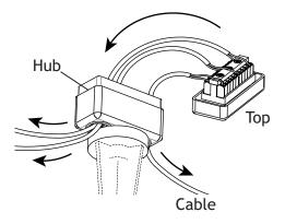
After all wires are connected, carefully pull the extra wire out of the bottom openings of the hub. Then, place the top back onto the hub.
