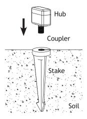
Thread the hub onto the stake and hand tighten until snug.
