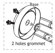
1. Pull the 2 holes grommet out of the base.
