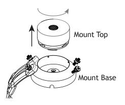
Twist and remove the mount top from the base.
