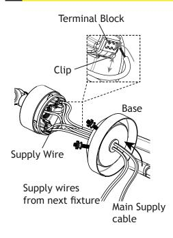
First, connect the wires from the fixture on the mount top. Use the following method.
