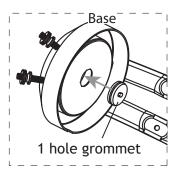
2. Push the 1 hole grommet into the center hole.
