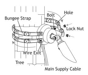
Place the wire in the wire exit slot making sure it is facing down. Then attach the mount to your desired tree. Wrap the bungee straps around the tree until a proper hole fits the tree size. Remove the lock nut and place the bolt through the hole on the bungee strap. Secure using the lock nut. Hand tighten until snug.
