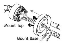
Place the mount base onto the mount top and rotate until they lock.
