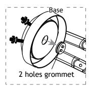
1. Pull the 2 holes grommet out of the base.
