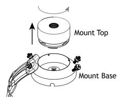
Twist and remove the mount top from the base.
