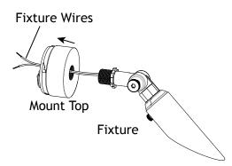
Pass the supply wires from the fixture through the mount top. Then thread the mount top onto the fixture and hand tighten until snug.
