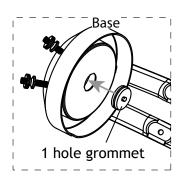
2. Push the 1 hole grommet into the center hole.
