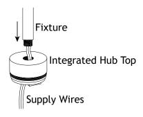
Pass the supply wires from the fixture through the integrated hub top. Thread the fixture onto the integrated hub top and hand tighten until snug.
