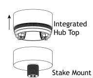
Loosen the integrated hub top and separate the integrated hub top from the stake mount.
