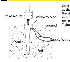
Clear away an area in the ground at the wireway slot on top of the stake. Lay the supply wires into the wireway slot and screw the stake mount on to the stake. Tighten until snug.
