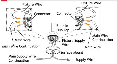
Insert the main supply wire continuation (if needed) and the main supply wire up through the bottom of the surface mount and strip the ends of both sets of supply wires.
