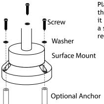
Place the surface mount onto the desired location and secure it with the screws. Tighten with a screwdriver. Nylon spacers are required when installing on trees.
