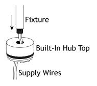
Pass the supply wires from the fixture through the built-in hub top. Thread the fixture onto the built-in hub top and hand tighten until snug.
