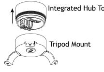
Loosen the integrated hub top and Integrated Hub Top separate the integrated hub top from the tripod mount.
