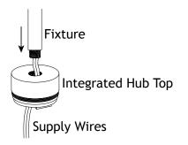
Pass the supply wires from the fixture through the integrated hub top. Thread the fixture onto the integrated hub top and hand tighten until snug.
