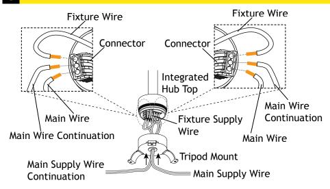
Insert the main supply wire continuation (if needed) and the main supply wire up through the bottom of the tripod mount and strip the ends of both sets of supply wires.
