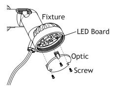
Loosen the screws, and remove the optic from the fixture.
