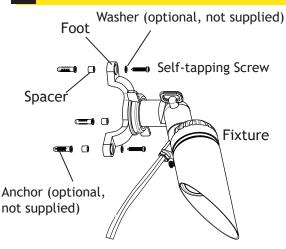
Determine the desired location for the fixture. Place the washers onto the self-tapping screws. Pass the self-tapping screws through the holes of the feet of fixture and spacers. Thread the self-tapping screws into the desired location to secure the fixture.
