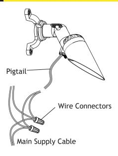
Strip both leads from the luminaire pigtail. Using two wire connectors (sold separately), connect the leads from the luminaire to the main supply cable leads.
