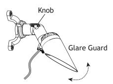
Loosen the knob and rotate the glare guard to your desired direction. Hand tighten the knob once your desired direction is achieved.
