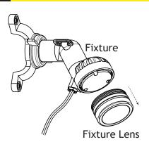
Turn the fixture lens counterclockwise and remove it from the fixture.
