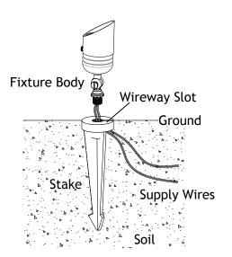
Clear away an area in the ground at the wireway slot on top of the stake. Lay the supply wires into the wireway slot and attach the fixture on to the stake. Tighten until snug.
