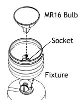
Insert MR16 bulb with the correct wattage and type marked on the fixture label and secure into place.
