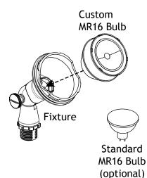
Use a custom or MR16 bulb (sold separately), with the correct wattage and type as marked on the luminaire label. Push the bulb onto the socket properly.
