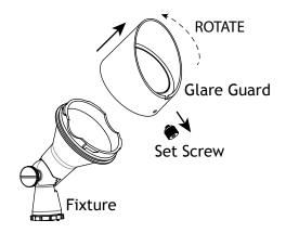
Loosen the set screw and remove it from the glare guard. Rotate the glare guard counter clockwise and remove it from the fixture. INSTALLATION INSTRUCTIONS
