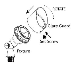
Thread the glare guard clockwise onto the fixture. Tighten the set screw back onto the glare.
