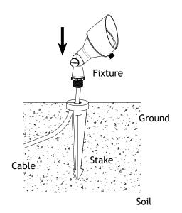
Pass the fixture wire through the center hole of the stake. Thread the fixture body onto the stake and hand tighten until snug.
