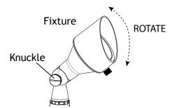
Loosen the knuckle and adjust the fixture to the desired orientation. Always tighten the knuckle after adjustment.
