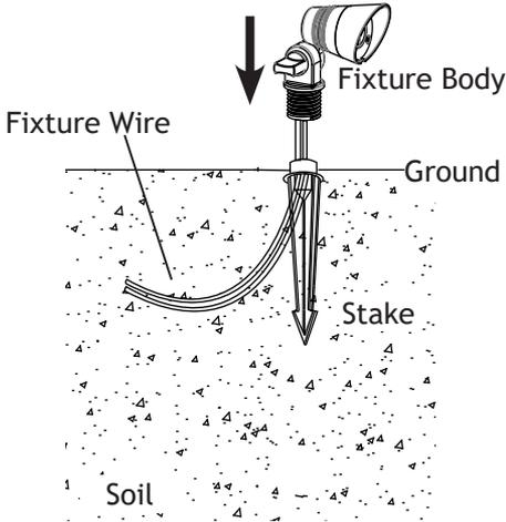
Clear away an area in the ground at the wireway slot on top of the stake. Lay the fixture wire into the wireway slot. Thread the fixture body onto the stake and hand tighten until snug.
