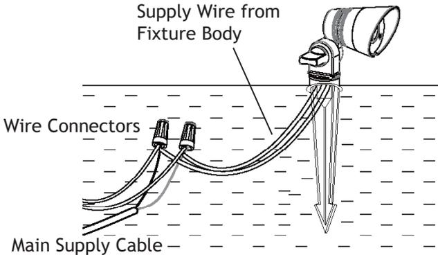
Strip both leads from the fixture body supply wires. Using two UL listed wire connectors (sold separately), connect supply wires from fixture body to the main supply cable leads.
