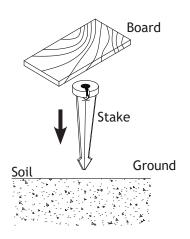
Determine the desired location for mounting the stake mount. Hammer the stake into the ground until flange of stake is flush to grade. To avoid damage to the stake, place a board on top of the stake while hammering.
