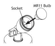
Insert MR11 Bulb with the correct wattage and type marked on fixture label and secure into place.
