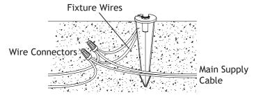
Strip both leads of the fixture wire. Using two UL listed wire connectors (sold separately), connect the leads from the fixture wire to the main supply cable leads.
