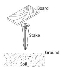
Determine the desired location for mounting the stake. Hammer the stake into the ground until flange of stake is flush to ground. To avoid damage to the stake, place a board on top of the stake while hammering.
