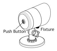
Change the light output of the fixture by using the push button on the back. The push button has the following options:
