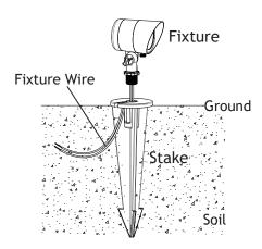
Pass the fixture wires through the open slot of the stake and thread the fixture onto the stake. Clear away an area in the ground to place the fixture wire.
