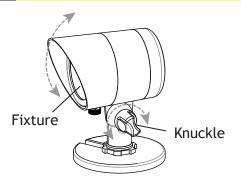
Adjust the fixture to your desired direction by loosening the knuckle.
